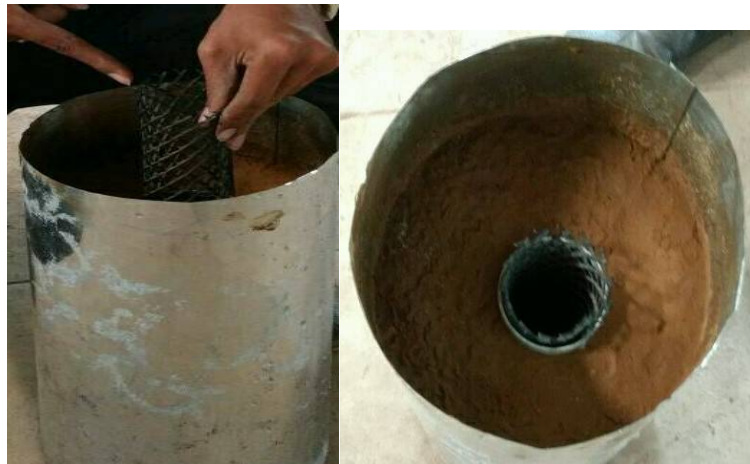
Fig.8 Placing of geo-grids
